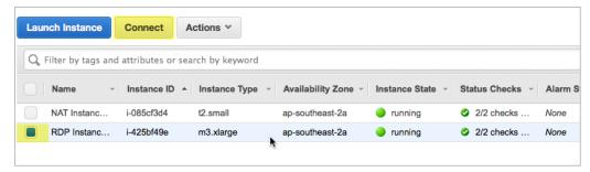
Figure 6: Connecting to the RDP instance
